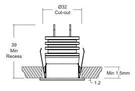
LED and optic position recessed by 10mm for reduced glare.
